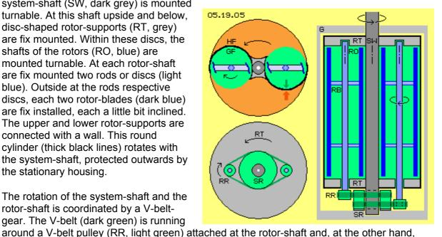
Relative to the glide-face, the air is moving by constant speed. The rotor-blades must not do accelerating or decelerating work. They just are rotating synchronous with the air all around. The blades are inclined a little bit, so they keep the whirlwinds local near the glide-faces all times. Picture 05.19.06 shows four situations of an animation, illustrating the movements of the cylinder and the rotor-blades (here e.g. with gear-relation 1:4).
