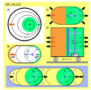
cylinder could achieve). A concentrated potential-vortex comes up. All other faces should be rough, so the flow at the opposite stick-face (HF, red) is much slower. In order to keep the air nearby resting at this area, even it could be protected by a 'palings-fence' (here marked by black points).
